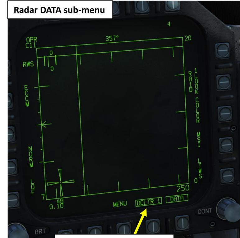
**Declutter** removes horizon line and velocity vector
