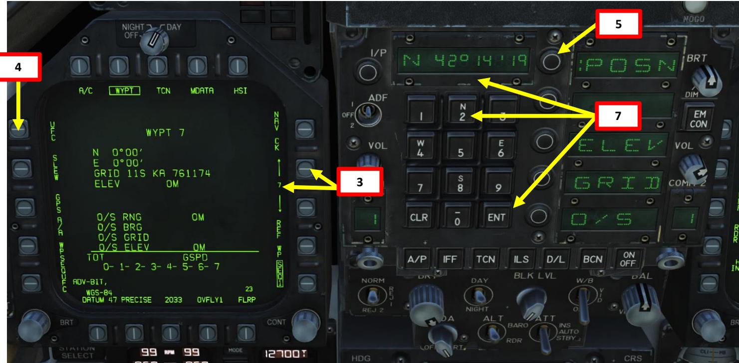
Coordinate format you input in the UFC is Degree, Minute, Seconds.
