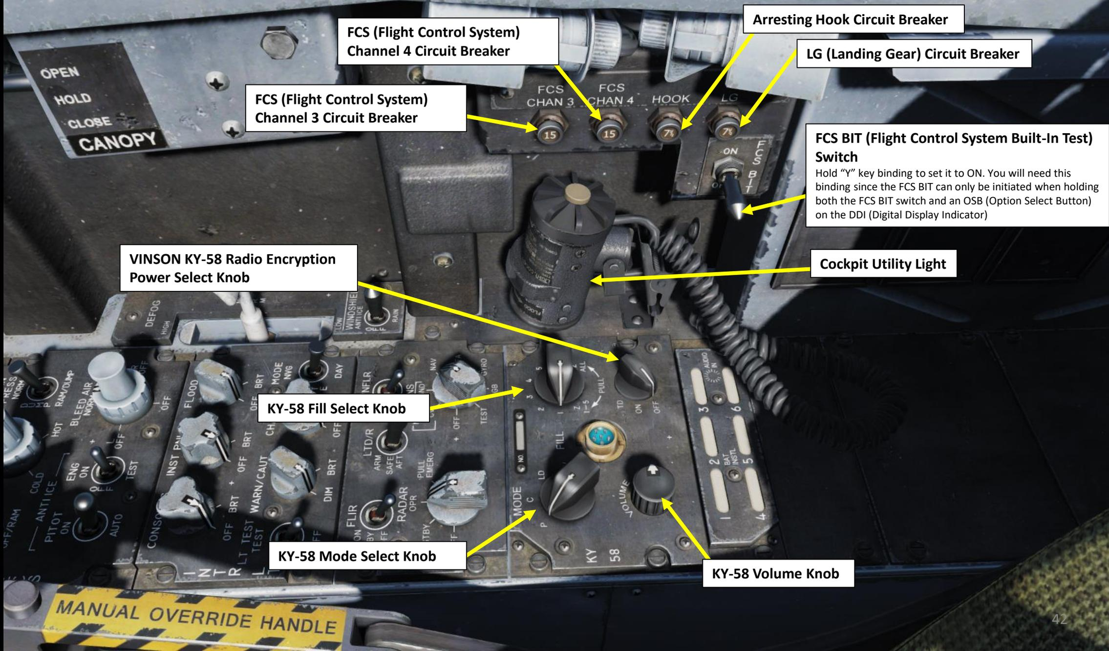
FCS (Flight Control System) Channel 4 Circuit Breaker
