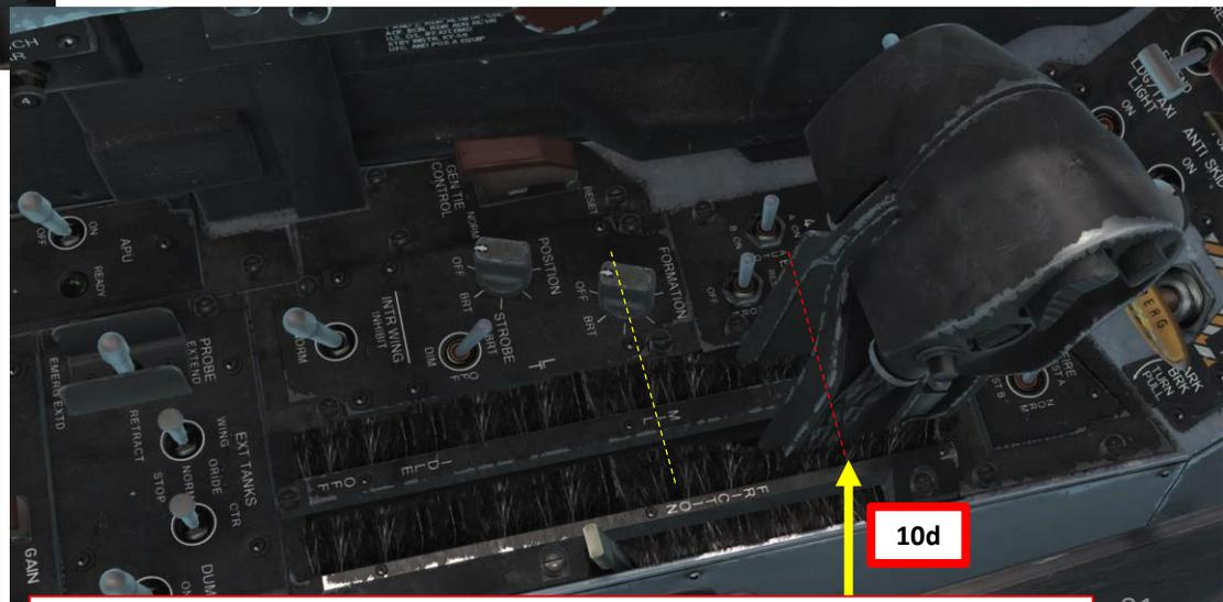
Afterburners not engaged, throttles stopped at MIL (Finger Lift Down)
