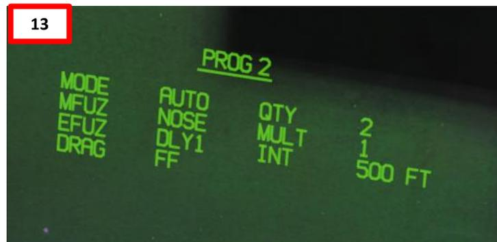
**Quantity (QTY).** Number of bombs to release, ranging from 1 to 30. When more than one bomb is selected, you must hold the Weapon Release Button down until all bombs in the salvo are released.
