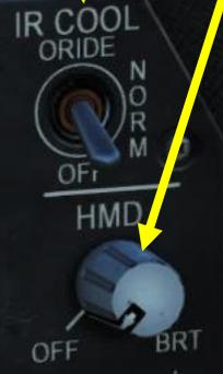
**HMD (Helmet-Mounted Display) Brightness Control Switch**
