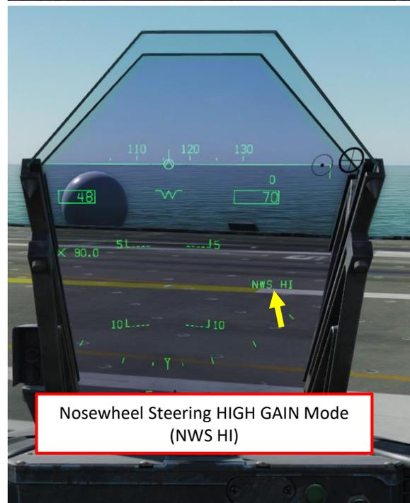
Nosewheel Steering HIGH GAIN Mode (NWS HI)
