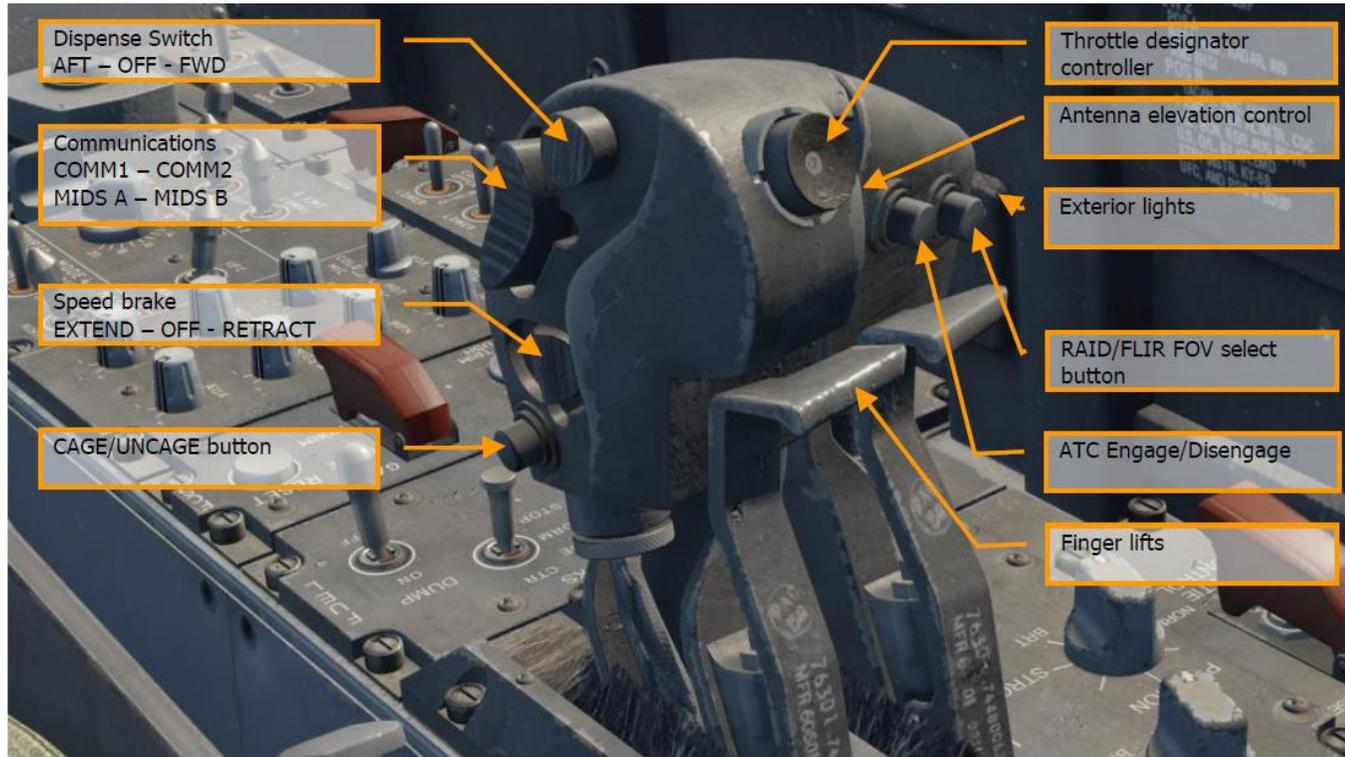
Finger lifts act as a stopper that prevents throttles from accidentally going from IDLE to OFF once engines are started. In order to shut down an engine, finger lifts are raised by pressing "0" for right throttle and "9" for left throttle.
