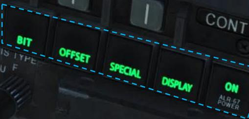
**ALR-67 RWR (Radar Warning Receiver) Control Buttons**
