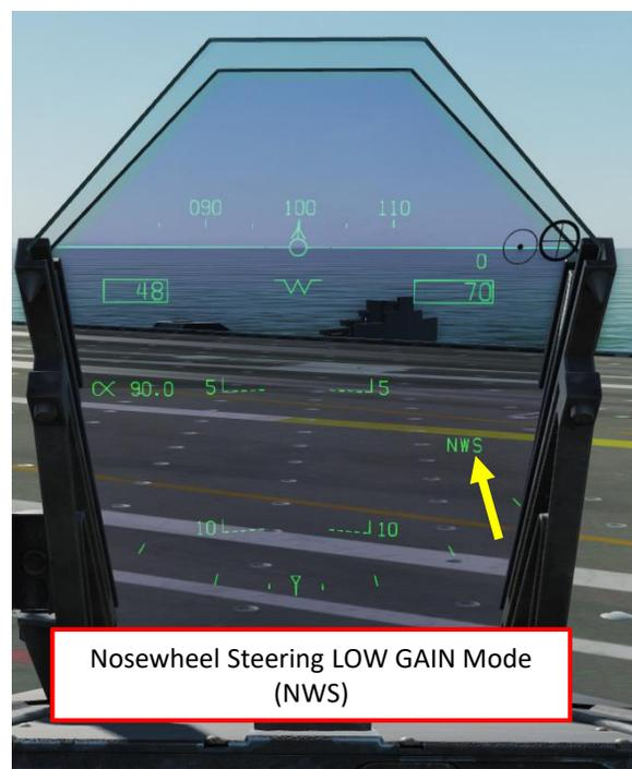
Nosewheel Steering LOW GAIN Mode (NWS)
