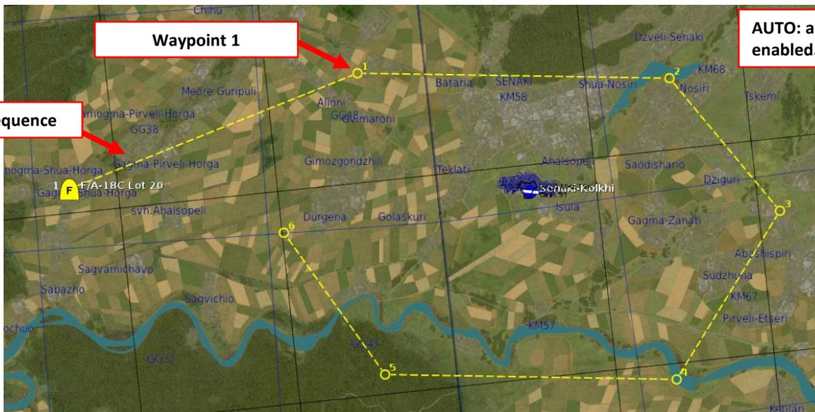
**AUTO:** automatic sequence steering to the next waypoint is enabled. WYPT must be selected as the navigation method
