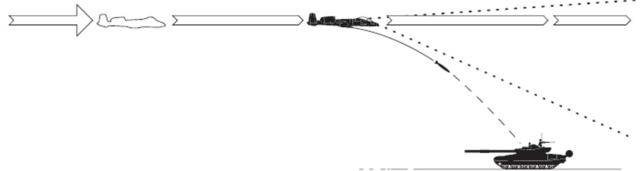
**CCRP: Continuously Computed Release Point**
